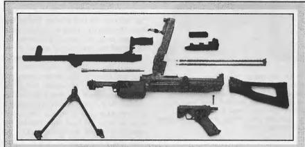
Production model SS-77 GPMG field stripped.
